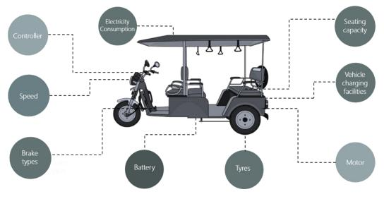
Figure 12: Components of an e-rickshaw
