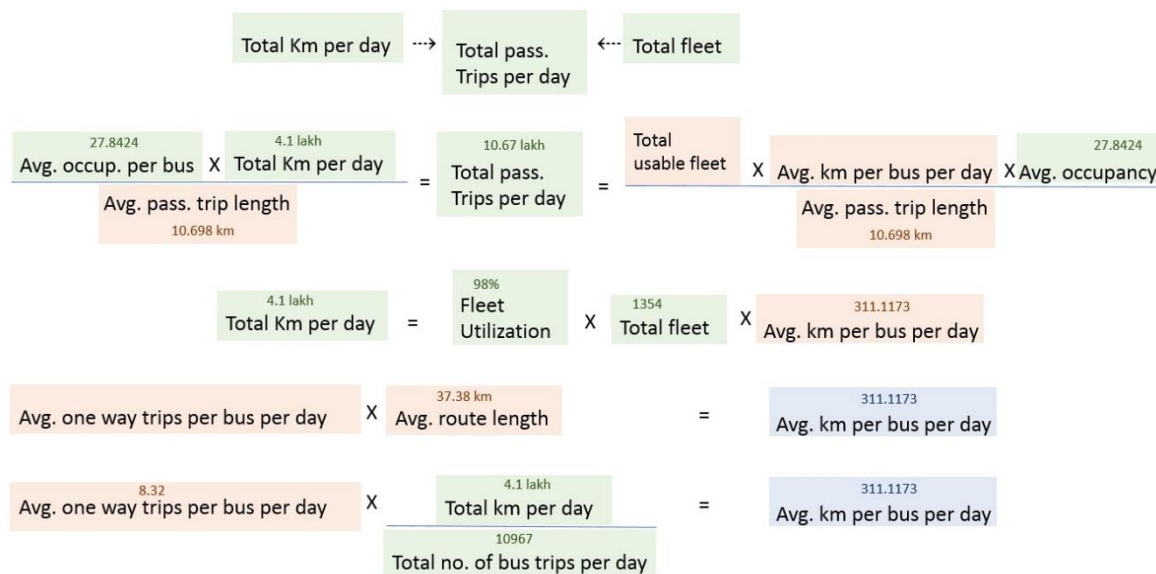
Figure 6 Estimation of Intracity fleet strength
