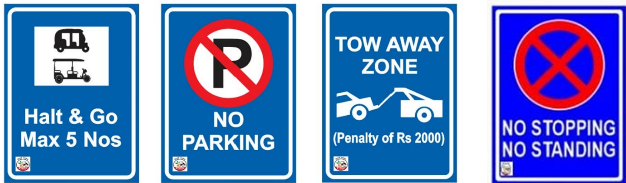
Figure 20: Sign board designs for the pilot stretch, to facilitate bus lane compliance
